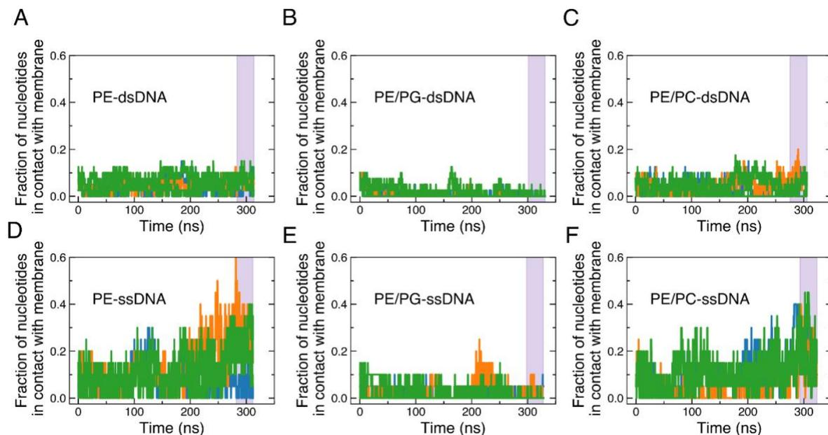
**Figure S5: Fraction of DNA in contact with membrane:** (A,B) Fraction of DNA nucleotides in contacts with the lipid bilayer as a function of simulation time. A contact was defined as a C3' atom of DNA backbone located within 5 Å of any non-hydrogen atoms of the membrane. The highlighted region indicates the part of the MD trajectories used to determine the average values reported in Figure 5D.
