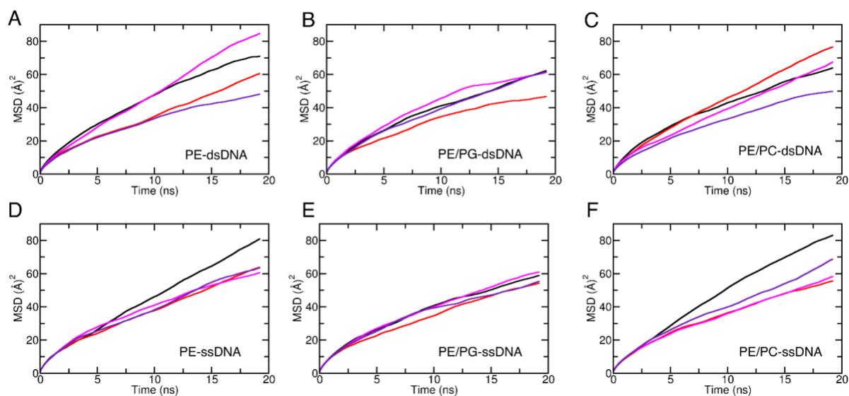
**Figure S9: Mean square displacement (MSD) of the cholesterol anchor as a function of simulation time.** The 20 ns MSD curves were extracted by averaging over 300 ns of the respective MD trajectories. The diffusion coefficients plotted in Figure 5H were computed as the least square fit to the MSD curves in the 7 to 20 ns range.
