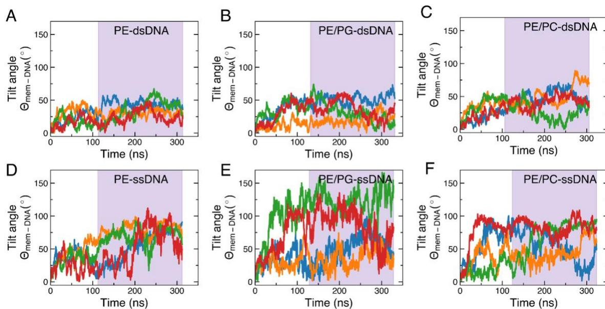
**Figure S4: Tilt angle versus simulation time.** The  $\theta_{\text{mem-DNA}}$  angle was defined as the angle between the bilayer normal and the line joining the CoM of the first and the last basepair of dsDNA or the second and the last nucleotide of ssDNA. The highlighted region indicates the part of the MD trajectories used to determine the average values reported in Figure 5C.
