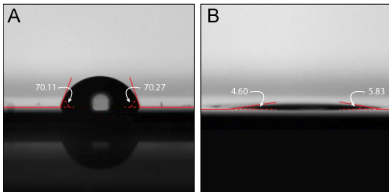
Figure S5. Contact angle measurements with 1M KCl, 10mM Tris, 1mM EDTA at pH 7.6 solution. Contact angle values (insets) of graphene (A) is observed to be much higher than that of dielectric  $\text{Al}_2\text{O}_3$  (B).
