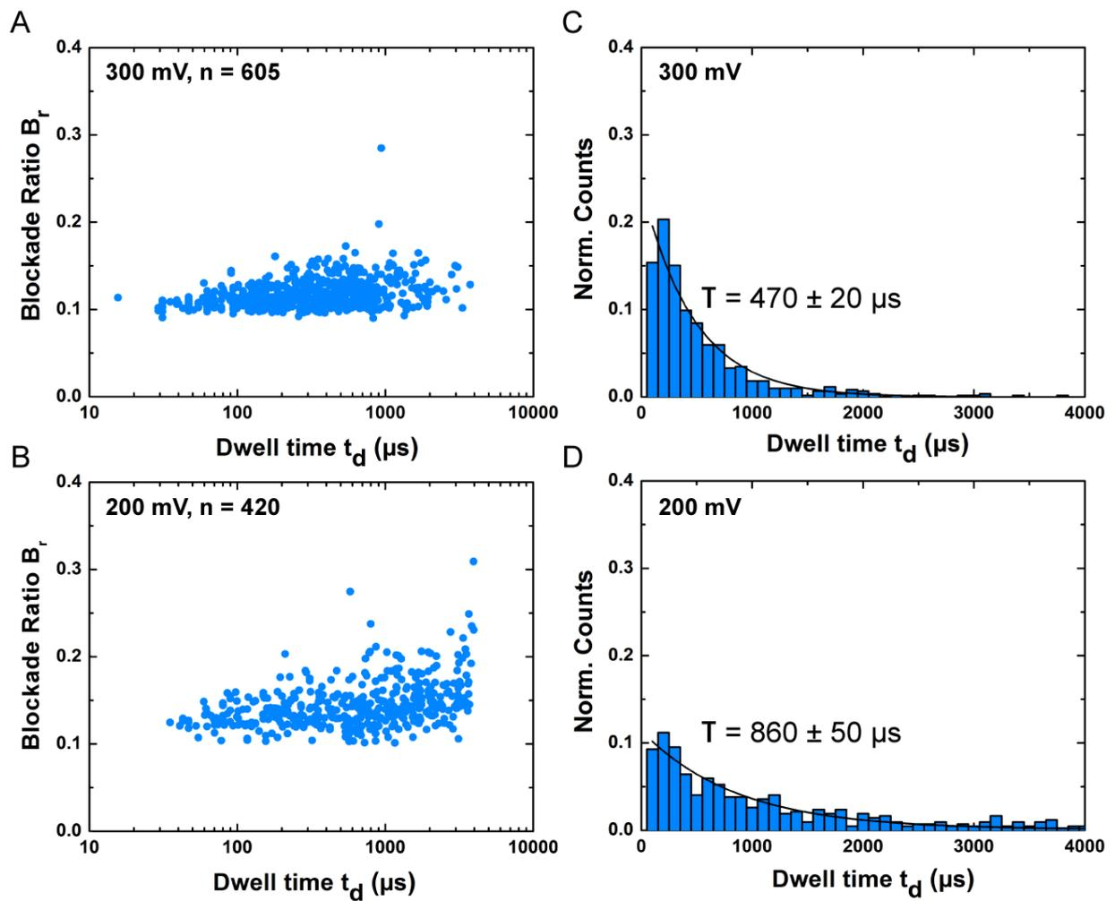
Figure S3. Scatter diagrams and translocation time histograms for a 4.0 nm nanopore in graphene-dielectric membrane at 300 mV and 200 mV used for 100nt ssDNA translocation experiments. The decreased translocation time at higher voltage (300 mV) indicates translocations of DNA molecules and not random collisions contributing to the data. All experiments were done in 1 M KCl, 10 mM Tris, 1 mM EDTA at pH 7.6.
